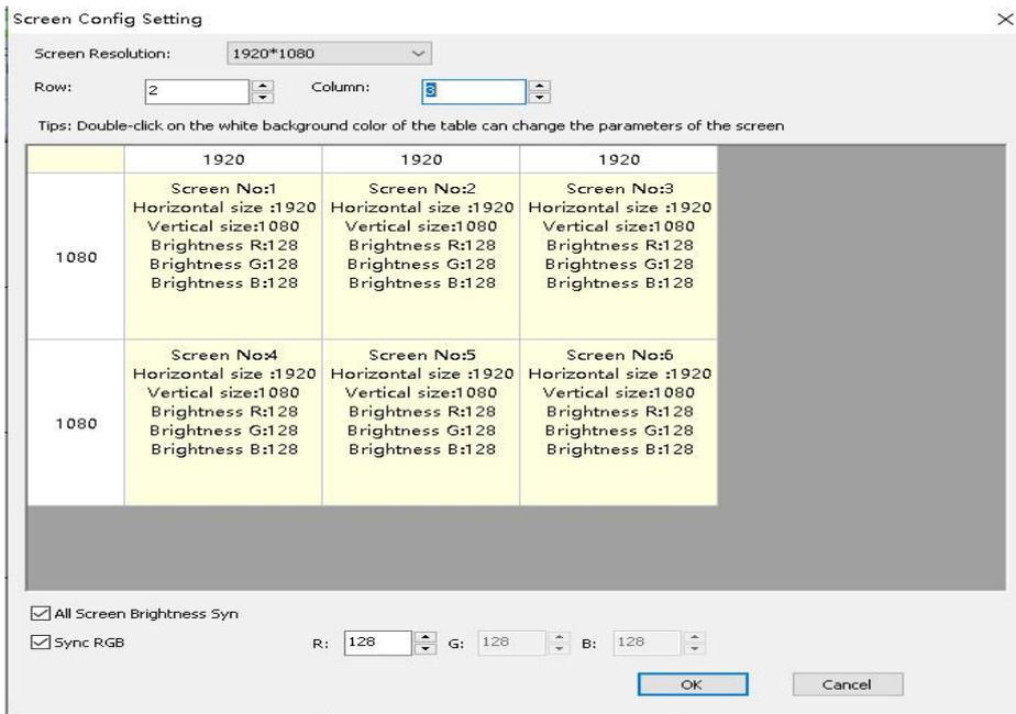
The "screen resolution" is the maximum resolution that can be output by each output port, and is generally greater than or equal to the resolution of each sending card or each display.
