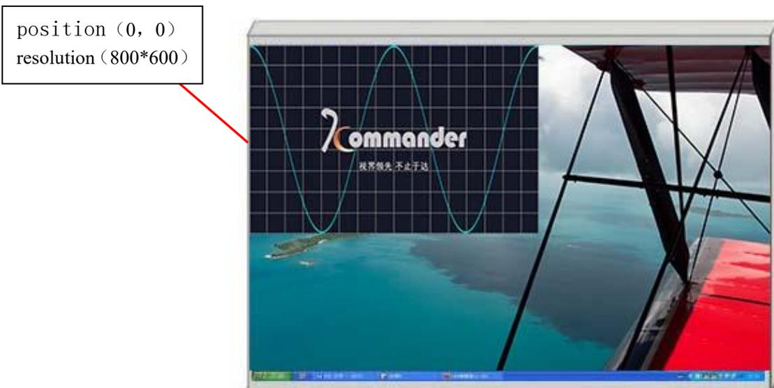
If you need to capture the blue flower area into a window and play it, you need to set the horizontal and vertical positions of the input scale of the window to 0, the horizontal size to 800, and the vertical size to 600. If the window is full screen, The effect on the screen is:
