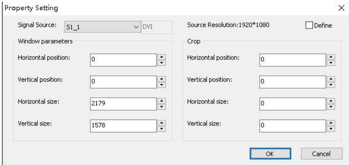
The property settings mainly include the following three items: signal source selection, picture parameters, and partial display.
